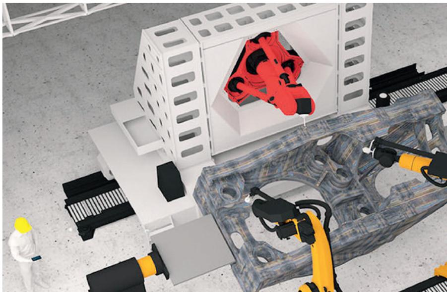
achieve such result, the deposition process will be based on wire + arc additive manufacture (WAAM). Another unique feature of the machine will be the capability for parallel manufacturing, featuring either multiple deposition heads or concurrent addition and subtraction processes.
